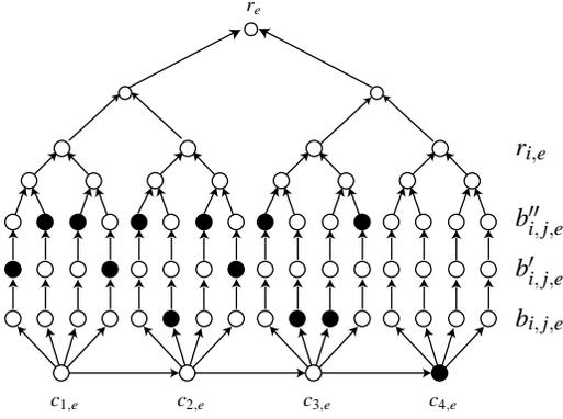
**Figure 4:** This figure shows a diagram of one ASPATH Protector using the postmodification mechanism. The grey circles represent the values of the ASPATH Protector that an AS receives in an UPDATE: the origin AS signs the first two ASNs with the one-time signature spanned by  $c_{1,e}$ , the second AS signs the first three ASNs with the one-time signature spanned by  $c_{2,e}$ , etc. We describe the details on which values are disclosed in the text.
