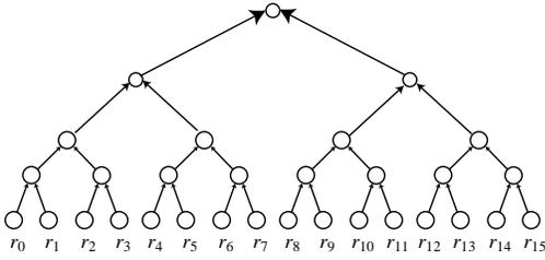
**Figure 3:** This figure shows a hash tree constructed over the epoch public keys (root nodes of 16 ASPATH protectors). The root node of this tree is the multi-epoch public key, which is signed with the prefix public key to form the multi-epoch certificate.
